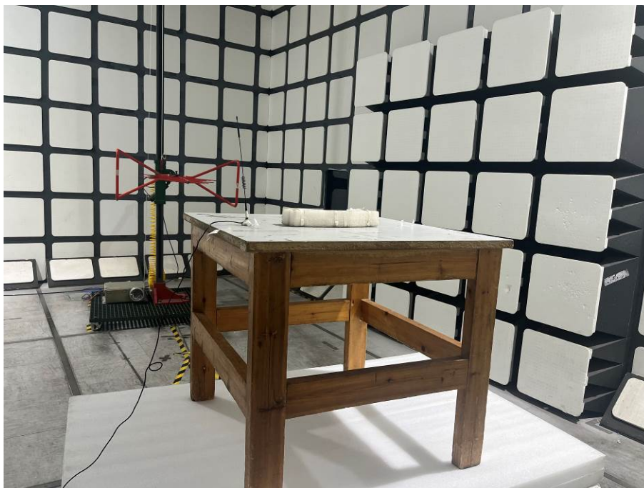
Radiated Spurious Emissions Test View (Above 1GHz)
